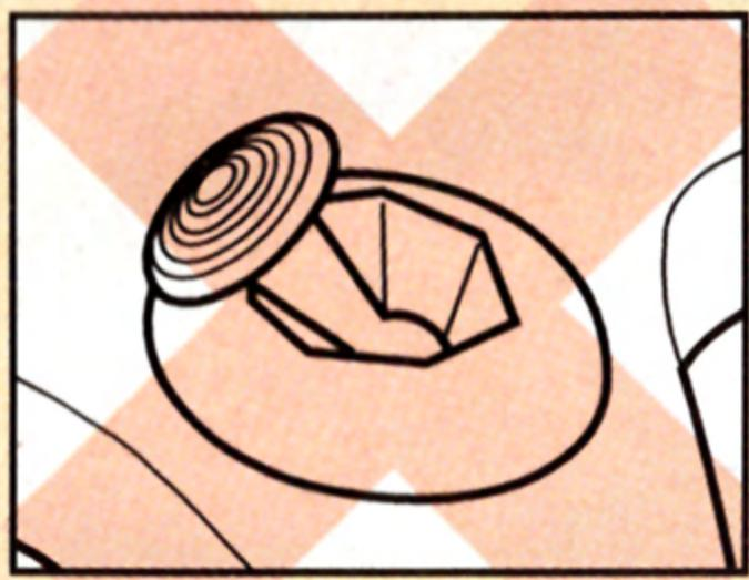
If the Control Stick is held at an angled position (as shown in the picture on the left) when the power is turned ON, this position will be set as neutral. This will cause games using the Control Stick to operate incorrectly.
